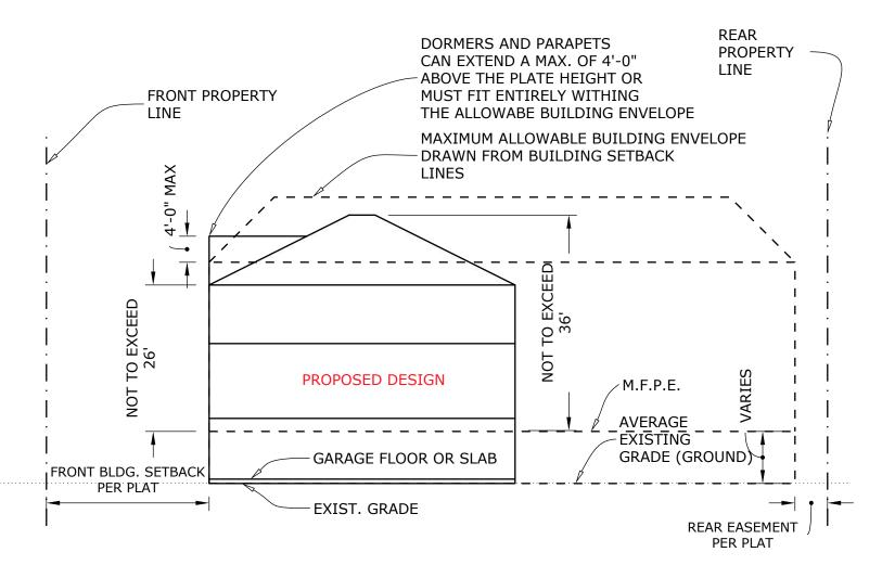
FIGURE 2 OF 3 - BUILDING AREA DIAGRAM - SIDE VIEW
