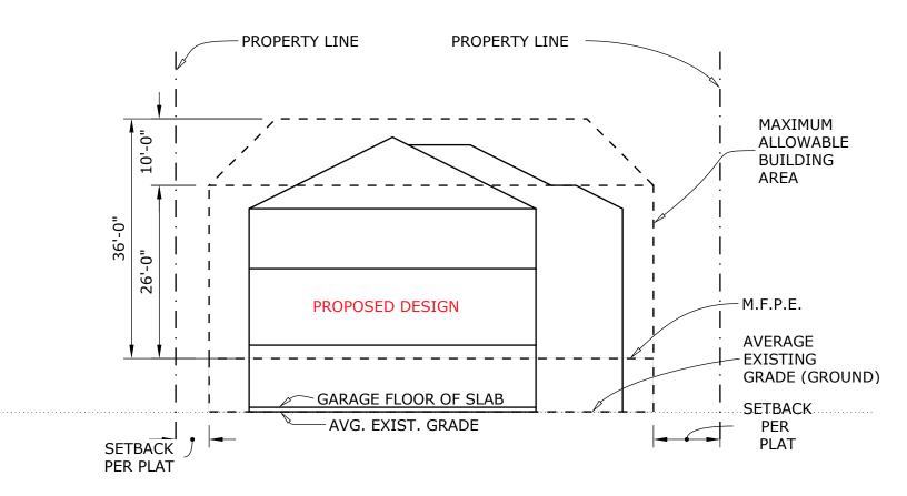
FIGURE 3 OF 3 - BUILDING AREA DIAGRAM - FRONT VIEW
