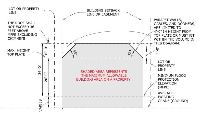
FIGURE 1 OF 3 - DIAGRAM OF BUILDABLE AREA
